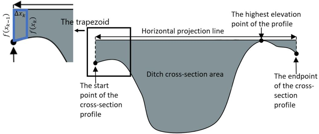
**Figure 4. Cross-section area definition.**
