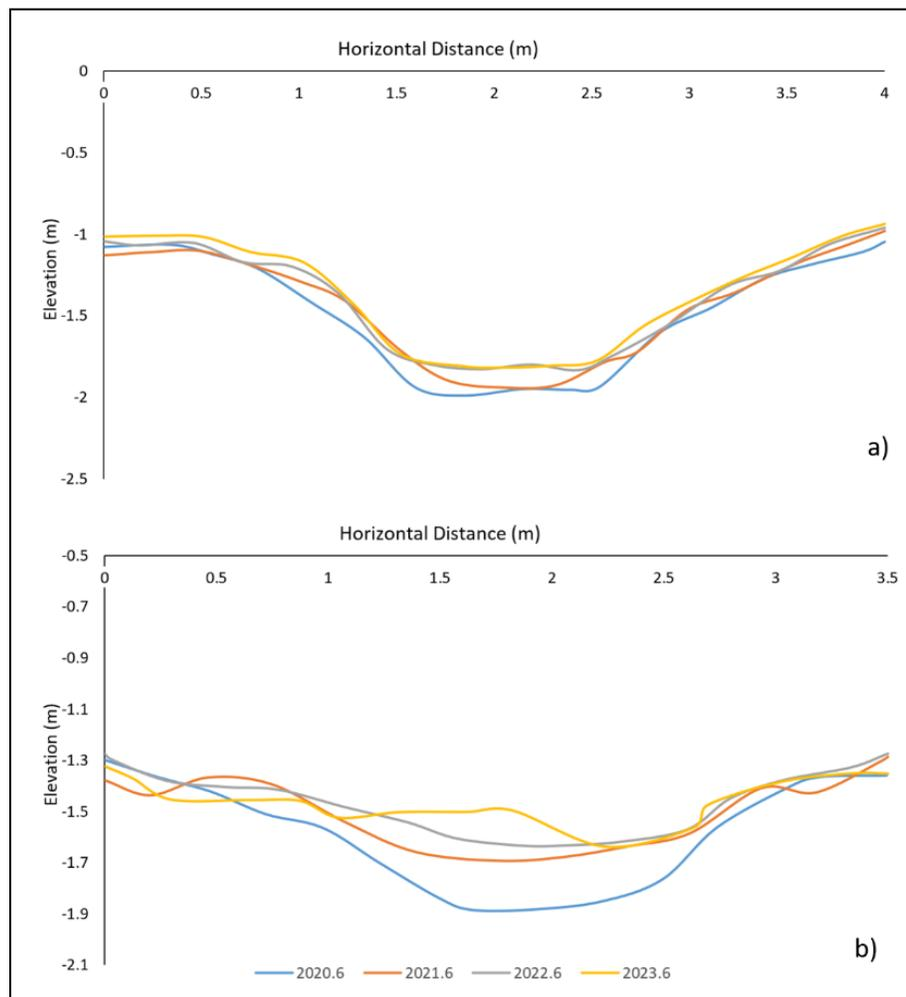
**Figure 9. (a) An example of getting shallower and narrower (the cross-section of the control one at 40 meters in YAM); (b) an example of getting shallower and broader (the cross-section of the ditch with a 2-m VFS at 500 meters in YAM).**
