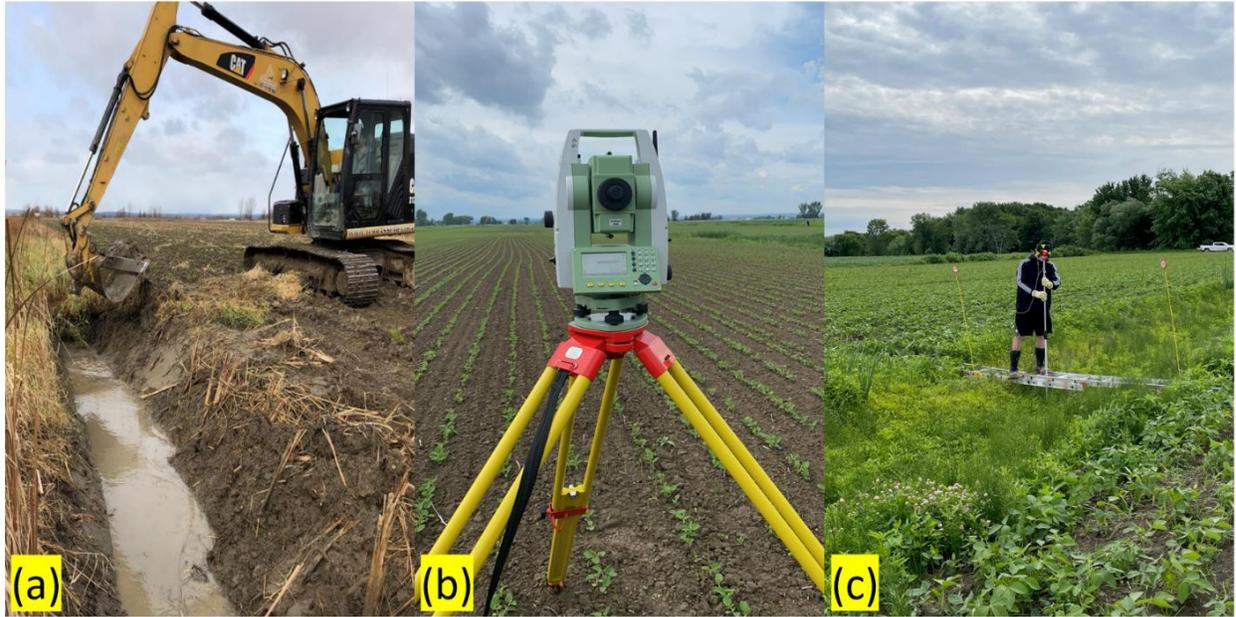
**Figure 3. (a) Ditch trenching. (b) the total station. (c) the progress of the measurement with the ladder.**
