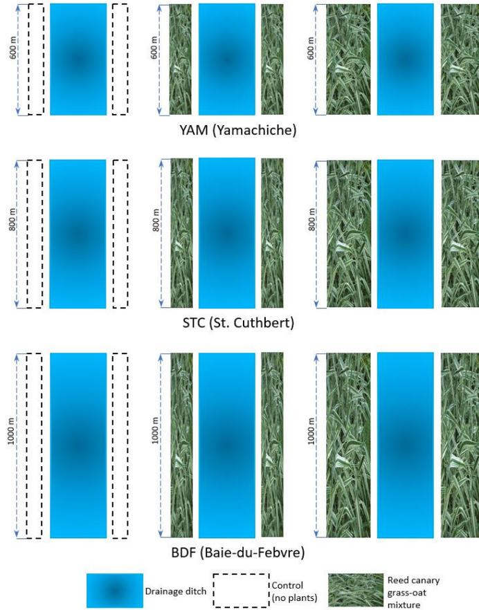
**Figure 2. Configuration of the vegetative filter strips (VFS) across three experimental sites, showing the arrangement of 2-meter and 4-meter-wide strips on both sides of the ditches.**
