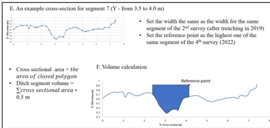
**Figure 7. Data processing pipeline. (A) an example of the bare ground point cloud of one ditch; (B) the raw bare ground point cloud of the selected plot; (C) an example of lowest point selection for one interval; (D) the cross-section view after points selection; (E) a cross-section example; (F) volume calculation.**
