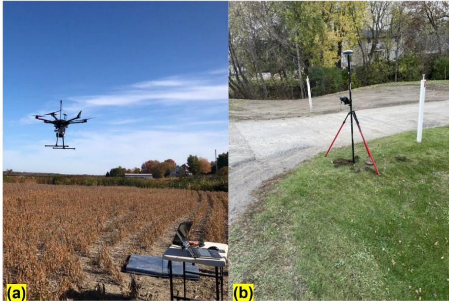
**Figure 5. (a) LiDAR sensor and its platform UAV; (b) the GNSS-base station setup.**
