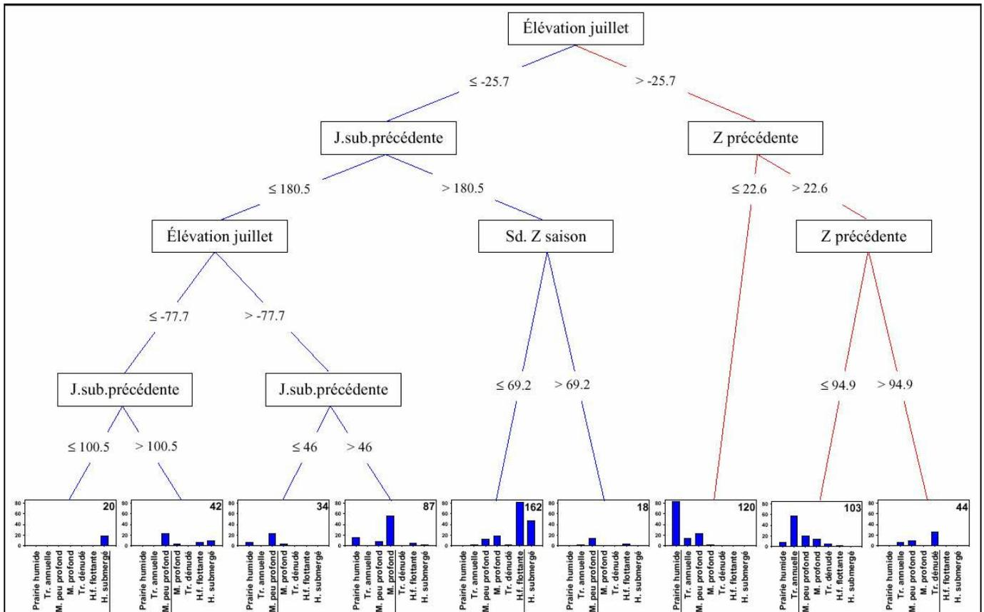
**Figure 12 Binary CART model (equation 12) allowing to predict wetland vegetation type from a combination of hydrological variables (from Hudon et al. 2003b).**
