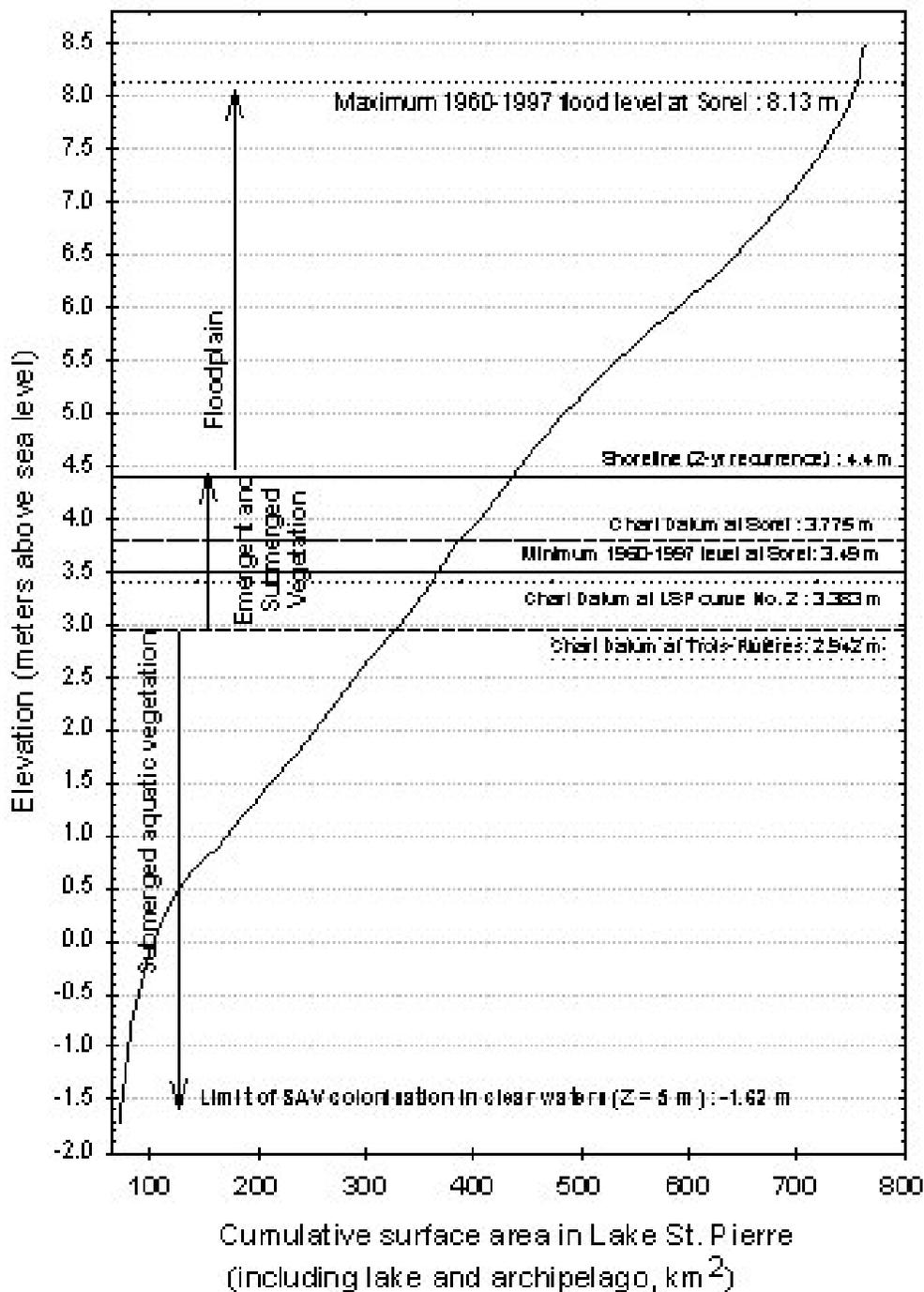
**Figure 7** Wetted surface area of Lake St. Pierre (km<sup>2</sup>) with increasing water level above sea level (ASL). Historical elevation thresholds defining the areas colonized by submerged aquatic vegetation (-1.67 to 2.94 m ASL), the belt of emergent and submerged vegetation (2.94 to 4.4 m ASL) and the floodplain (4.4 to 8.13 m ASL) are indicated.
